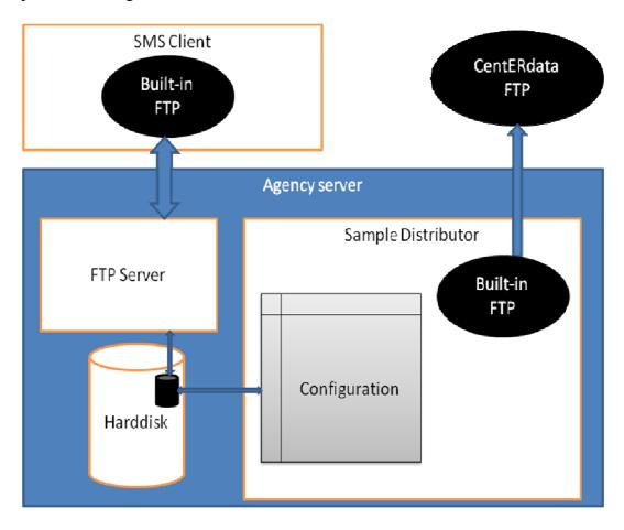
Figure 3.4: System overview for automatic FTP-synchronization
